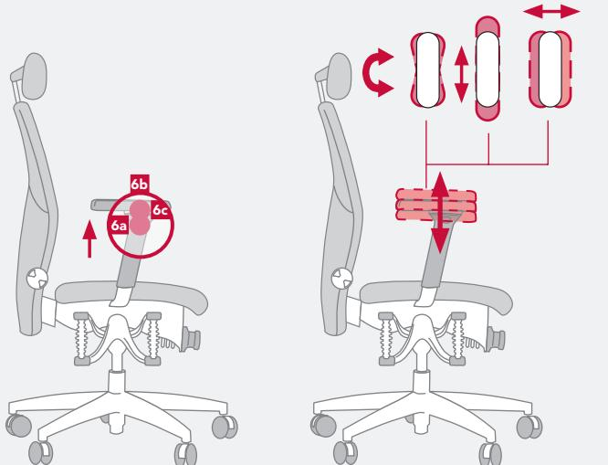
The armrest can be adjusted in height in order to relieve the shoulder and neck muscles. Adapt the height so that no tension subsists in the shoulder. In addition to that you can adjust the armrest pads to the morphology of the thorax, arms and forearms in a large variety of positions.
